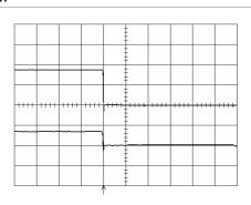
Shut-down enabled by disconnecting V<sub>I</sub> at:  $T_{\rm ref}$  = +25°C, I<sub>O</sub> = 22 A resistive load, V<sub>I</sub> = 3.3 V.
