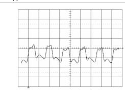
Output voltage ripple (20mV/div.) at:  $T_{ref} = +25^{\circ}C$ ,  $I_{O} = 22$  A resistive load,  $V_{I} = 3.3$  V. Time scale: 2 µs/div.
