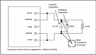
Output ripple and noise test setup
