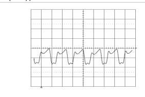
Output voltage ripple (20mV/div.) at:  $T_{ref} = +25^{\circ}C$ ,  $I_{O} = 22$  A resistive load,  $V_{I} = 3.3$  V. Time scale: 2 µs/div.
