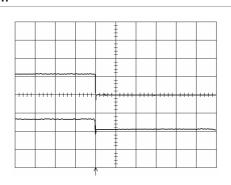
Shut-down enabled by disconnecting V<sub>I</sub> at:  $T_{ref} = +25^{\circ}\text{C}$ ,  $I_{O} = 22$  A resistive load,  $V_{I} = 3.3$  V.
