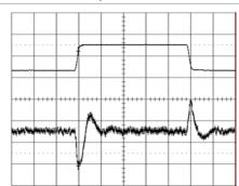
Output voltage response to load current step- Top trace: output voltage (50mV/div.). change (11-22-11 A) at: Bottom trace: load current (10 A/div.).  $T_{ref} = +25^{\circ}C, \ V_{l} = 3.3 \ V.$  Time scale: 0.1 ms/div..
