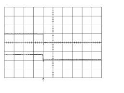
Top trace: output voltage (0.5 V/div.). Bottom trace: input voltage (2 V/div.). Shut-down enabled by disconnecting V<sub>I</sub> at:  $T_{ref} = +25^{\circ}\text{C}$ ,  $I_{O} = 22$  A resistive load,  $V_{I} = 3.3$  V. Top trace: output voltage (1.0 V/div.). Bottom trace: input voltage (2 V/div.). Time scale: 5.0 ms/div..
