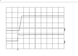
Start-up enabled by connecting V<sub>I</sub> at:  $T_{ref} = +25^{\circ}C$ ,  $I_{O} = 22$  A resistive load,  $V_{I} = 3.3$  V.
