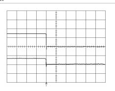
Shut-down enabled by disconnecting V<sub>I</sub> at:  $T_{ref} = +25^{\circ}\text{C}$ ,  $I_{O} = 22$  A resistive load,  $V_{I} = 3.3$  V.
