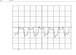
Output voltage ripple (20mV/div.) at:  $T_{ref} = +25^{\circ}C$ ,  $I_{O} = 22$  A resistive load,  $V_{I} = 3.3$  V. Time scale: 2 µs/div.
