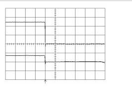
Shut-down enabled by disconnecting V<sub>i</sub> at:  $T_{\rm ref}$  = +25°C, I<sub>O</sub> = 22 A resistive load, V<sub>i</sub> = 3.3 V.
