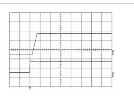
Start-up enabled by connecting V<sub>I</sub> at:  $T_{ref} = +25^{\circ}C$ ,  $I_{O} = 22$  A resistive load,  $V_{I} = 3.3$  V.
