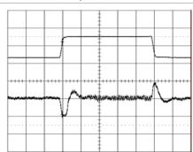
Output voltage response to load current step- Top trace: output voltage (100mV/div.). change (11-22-11 A) at: Bottom trace: load current (10 A/div.).  $T_{ref} = +25^{\circ}\text{C}, \ V_{l} = 3.3 \text{ V}.$  Time scale: 0.1 ms/div..
