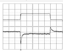
Output voltage response to load current step- Top trace: output voltage (100mV/div.). change (11-22-11 A) at: Bottom trace: load current (10 A/div.).  $T_{ref} = +25^{\circ}\text{C}, \ V_{l} = 3.3 \text{ V}.$  Time scale: 0.1 ms/div..
