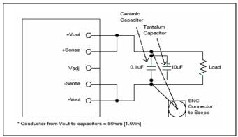
Output ripple and noise test setup
