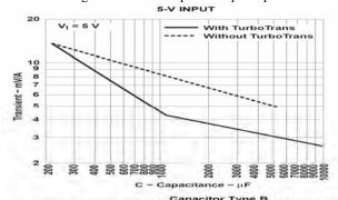
Capacitor Type B,  $1000 < C(\mu F) \times ESR(m\Omega) \le 5000$  (e.g. Polymer-Tantalum)
