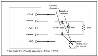
Output ripple and noise test setup
