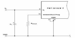
Undervoltage Lockout Adjustment Resistor Placement
