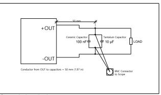
Output ripple and noise test setup
