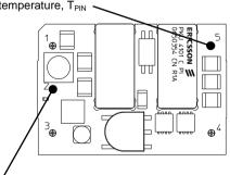
Pin 2 for measurement of maximum product temperature, T<sub>PRODUCT</sub>
