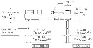
$\label{eq:total_total} \ensuremath{\mathsf{TOP}} \ensuremath{\,\mathsf{VIEW}}$  Pin positions according to the recommended footprint
