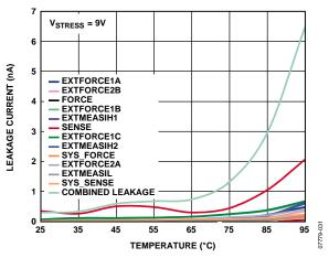
Figure 19. Leakage Current vs. Temperature (Force and Combined Leakage),  $V_{STRESS} = 9 V$
