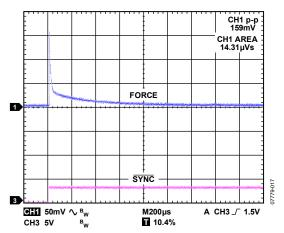
Figure 32. Range Change 25 mA to EXTFORCE2, Safe Mode, 25 mA  $I_{\rm LOAD}$ , 10  $\mu F$  Load
