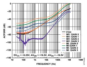
Figure 49. ACPSRR of AV<sub>SS</sub> vs. Frequency
