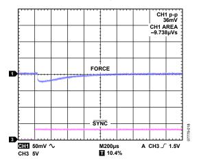
Figure 33. Range Change EXTFORCE2 to 25 mA, Safe Mode, 25 mA  $_{\rm LOAD}$ , 10  $\mu{\rm F}$  Load
