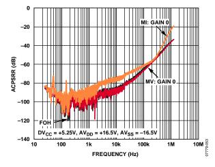
Figure 52. ACPSRR of HCAV<sub>SS</sub>X vs. Frequency
