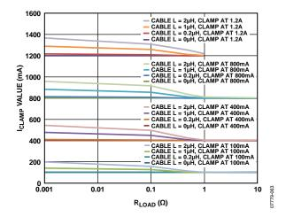
Figure 53.  $I_{CLAMP}$  Value vs.  $R_{LOAD}$  – Cal at 10hm
