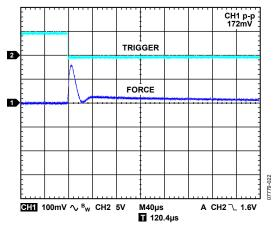
Figure 37. Safe Mode 80% to 10%, EXTFORCE2 Range, 10 μF Load
