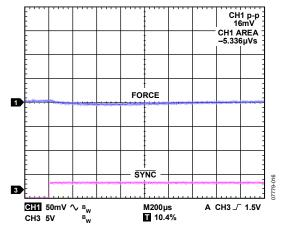
Figure 31. Range Change 25 mA to 2.5 mA, Safe Mode, 2.5 mA I<sub>LOAD</sub>, 10 μF Load
