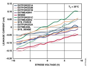
Figure 20. Leakage Current vs. Stress Voltage
