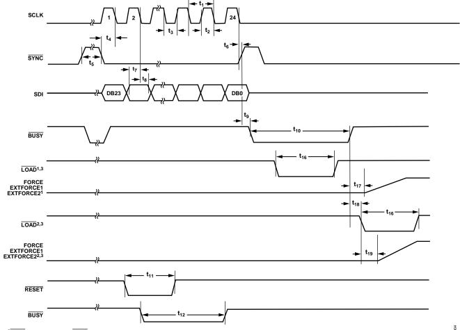
$^1 \underline{\text{LOAD}}$  ACTIVE DURING  $\underline{\text{BUSY}}.$   $^2 \underline{\text{LOAD}}$  ACTIVE AFTER  $\underline{\text{BUSY}}.$   $^3 \underline{\text{LOAD}}$  FUNCTION IS AVAILABLE VIA CLEN OR  $\overline{\text{HW}\_\text{INH}}$  AS DETERMINED BY DPS REGISTER 2.
