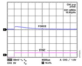
Figure 30. Range Change 2.5 mA to 25 mA, Safe Mode, 2.5 mA I<sub>LOAD</sub>, 10 μF Load
