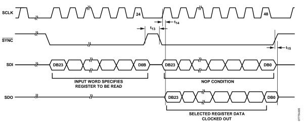
Figure 5. SPI Read Timing
