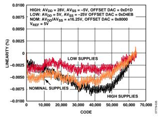
Figure 12. Measure Current Linearity vs. Code (MEASOUT Gain = 1, MI Gain = 20),  $T_J = 25$ °C
