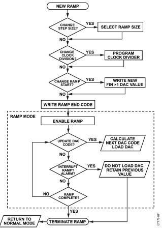
Figure 59. Flow Chart for Ramp Function
