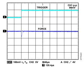
Figure 36. Autocompensation Mode 10% to 90% I<sub>LOAD</sub> Change, EXTFORCE2 Range, 10 µF Load
