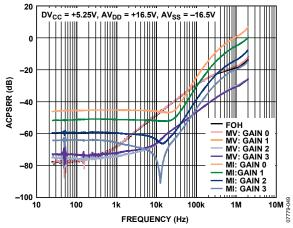
Figure 48. ACPSRR of AV<sub>DD</sub> vs. Frequency
