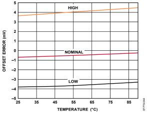
Figure 29. MV Offset Error vs. Temperature, MEASOUT Gain = 0.2
