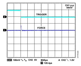
Figure 35. Autocompensation Mode 90% to 10% I<sub>LOAD</sub> Change, EXTFORCE2 Range, 10 μF Load
