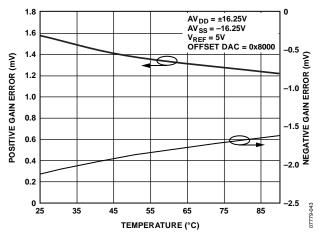
Figure 24. FV Gain Error vs. Temperature
