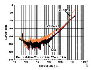
Figure 51. ACPSRR of  $HCAV_{DD}x$  vs. Frequency
