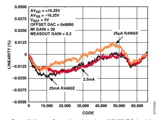
Figure 17. Measure Current Linearity vs. I<sub>RANGE</sub> (MEASOUT Gain = 0.2, MI Gain = 20)
