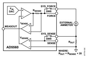
Figure 58. Measure Current Calibration
