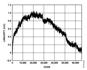
Figure 8. Force Voltage Linearity vs. Code,  $V_{REF} = 5 V$ , No Load
