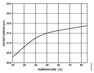
Figure 25. FV Offset Error vs. Temperature
