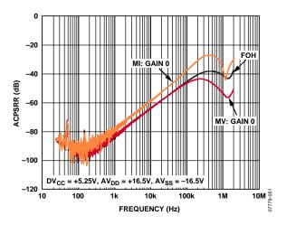
Figure 50. ACPSRR of  $DV_{CC}$  vs. Frequency
