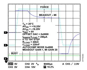
Figure 40. Transient Response FVMI Mode, ±250 μA Range, Autocompensation Mode
