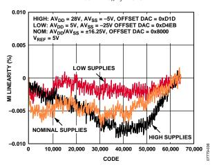
Figure 13. Measure Current Linearity vs. Code (MEASOUT Gain = 1, MI Gain = 10)
