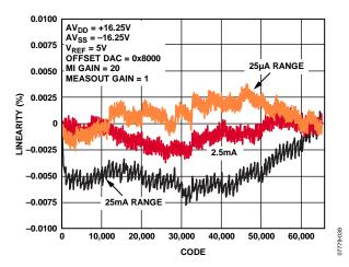
Figure 16. Measure Current Linearity vs.  $I_{RANGE}$  (MEASOUT Gain = 1, MI Gain = 20)
