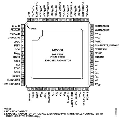
Figure 6. TQFP\_EP Pin Configuration
