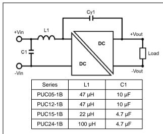
Based on different applications or PCB layout conditions, the EMI requirement may be varied. Recommend to reserve Cy1 for better EMI performance. Depending on the different requirement of end users, the value of Cy1 could be adjusted from 33pF to 470pF.
