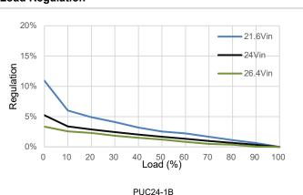
Output voltage with load variation vs. load current at T<sub>P1</sub> = +25°C
