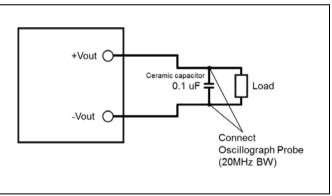
Output ripple and noise test setup
