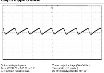
Trace: output voltage (50 mV/div.). Time scale: (10 µs/div.). 20 MHz bandwidth filter +0.1 µF
