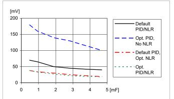
Load transient peak voltage deviation vs. external capacitance. Step-change (3-9-3 A). Parallel coupling of capacitors with 470  $\mu$ F/10 m $\Omega$ , T<sub>P1</sub> = +25°C. V<sub>I</sub>=12 V, V<sub>0</sub>=3.3 V, f\_{sw}=320 kHz, di/dt=2 A/µs
