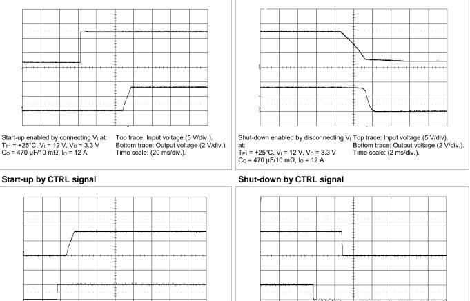
Start-up by enabling CTRL signal at:  $T_{P1}$  = +25°C, V<sub>I</sub> = 12 V, V<sub>O</sub> = 3.3 V  $C_0$  = 470 µF/10 mΩ, I<sub>O</sub> = 12 A
