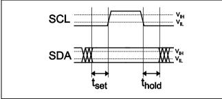
Setup and hold times timing diagram
