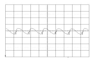
Output voltage ripple at: TP1 = +25°C, Trace: output voltage (10 mV/div.).  $V_{I} = 12 V, C_{O} = 470 \mu F/10 m\Omega$ Time scale: (2 µs/div.). I<sub>0</sub> = 12 A
