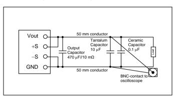
Output ripple and noise test set-up.
