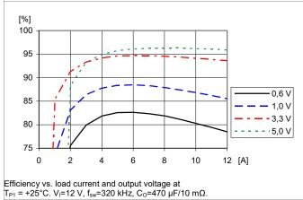
Efficiency vs. Output Current and Switch Frequency
