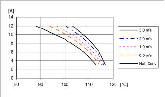
Available load current vs. ambient air temperature and airflow at V\_0=1.0 V, V\_I=12 V. See Thermal Consideration section.
