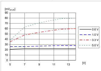
Output voltage ripple V\_{pk-pk} at: T\_{P1} = +25°C, C\_0=470  $\mu F/10$  mΩ, I\_0 =12 A.
