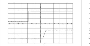
Start-up enabled by connecting V<sub>I</sub> at:  $T_{P1}$  = +25°C, V<sub>I</sub> = 12 V, V<sub>0</sub> = 3.3 V  $C_0$  = 470  $\mu F/10$  mΩ, I<sub>0</sub> = 12 A
