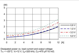
Power Dissipation vs. Output Current and **Switch Frequency**
