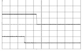
Shut-down enabled by disconnecting V<sub>I</sub> Top trace: output voltage (2 V/div). at: Bottom trace: CTRL signal (2 V/div.).  $T_{P1} = +25^{\circ}C, V_{I} = 12 \text{ V}, V_{O} = 3.3 \text{ V} \\ C_{O} = 470 \ \mu\text{F}/10 \ \text{m}\Omega, I_{O} = 12 \text{ A}$
