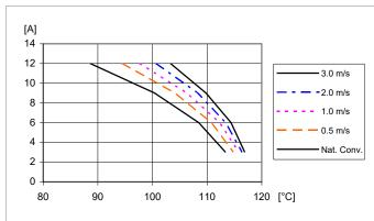
Available load current vs. ambient air temperature and airflow at  $V_0=0.6 V$ ,  $V_1=12 V$ . See Thermal Consideration section.
