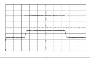
Output voltage response to load current stepchange (3-9-3 A) at: T<sub>P1</sub> = +25°C, V<sub>1</sub> = 12 V, V<sub>0</sub> =3.3 V di/dt=2 A/μs, f<sub>sw</sub>=320 kHz, C<sub>0</sub>=470 μF/10 mΩ
