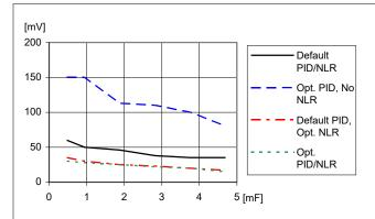
Load transient peak voltage deviation vs. external capacitance. Step-change (3-9-3 A). Parallel coupling of capacitors with 470  $\mu$ F/10 m $\Omega$ , T<sub>P1</sub> = +25°C. V<sub>I</sub>=12 V, V<sub>O</sub>=1.0 V, f<sub>sw</sub>=320 kHz, di/dt=2 A/ $\mu$ s
