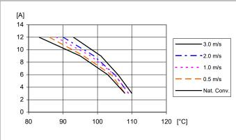
Available load current vs. ambient air temperature and airflow at Vo=3.3 V, VI = 12 V. See Thermal Consideration section.
