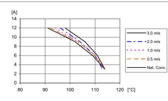
Available load current vs. ambient air temperature and airflow at  $V_0=0.6$  V,  $V_1=12$  V. See Thermal Consideration section.
