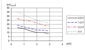
Output voltage ripple V<sub>pk-pk</sub> at: T<sub>P1</sub> = +25°C, V<sub>I</sub> = 12 V. I<sub>O</sub> = 12 A. Parallel coupling of capacitors with 470  $\mu$ F/10 mΩ,
