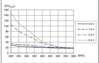
Output voltage ripple V<sub>pk-pk</sub> at: T<sub>P1</sub> = +25°C, V<sub>1</sub> = 12 V, C<sub>O</sub>=470 μF/10 mΩ, Io = 12 A resistive load. Default configuration except changed frequency. Load transient vs. Switching frequency
