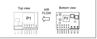
Temperature positions and air flow direction.
