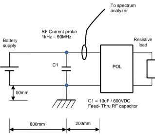
Conducted EMI test set-up
