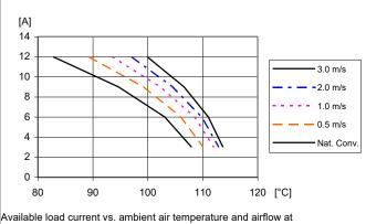
Available load current vs. ambient air temperature and airflow at  $V_0=3.3 \text{ V}$ ,  $V_1=12 \text{ V}$ . See Thermal Consideration section.
