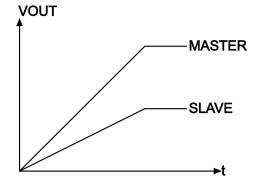
Illustration of Ratiometric Voltage Tracking
