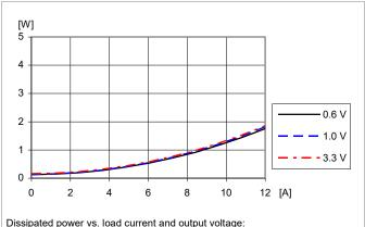
Dissipated power vs. load current and output voltage:  $T_{P1}$  = +25°C. VI=5 V,  $f_{sw}$ =320 kHz, C0=470  $\mu$ F/10 m $\Omega$
