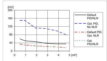
Load transient peak voltage deviation vs. external capacitance.  $\begin{array}{l} \label{eq:step-change} \end{tabular} \end{tabular}$
