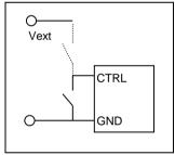
The product is equipped with a remote control function, i.e., the CTRL pin. The remote control can be connected to either the primary negative input connection (GND) or an external voltage (Vext), which is a 3-5.5 V positive supply voltage in accordance to the SMBus Specification version 3.0.
