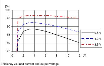
T<sub>P1</sub> = +25°C. V<sub>i</sub>=5 V,  $f_{sw}$ =320 kHz, C<sub>0</sub>=470 µF/10 mΩ.
