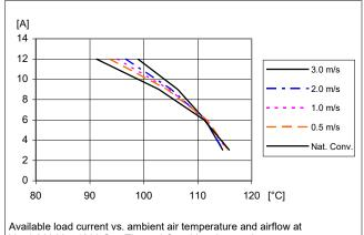
Available load current vs. ambient air temperature and airflow at V\_0=1.0 V, V\_1=12 V. See Thermal Consideration section.
