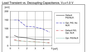
Load transient peak voltage deviation vs. decoupling capacitance. Step-change (3-9-3 A). Parallel coupling of capacitors with 470  $\mu F/10~m\Omega,$ T<sub>P1</sub> = +25°C. V<sub>I</sub>=12 V, V<sub>O</sub>=1.0V, f<sub>sw</sub>=320 kHz, di/dt=2 A/µs
