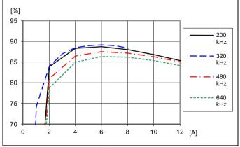
Efficiency vs. load current and switching frequency at  $T_{P1} = +25^{\circ}C$ . V<sub>1</sub>=12 V, V<sub>0</sub>=3.3V, C<sub>0</sub>=470 µF/10 m $\Omega$ Default configuration except changed frequency
