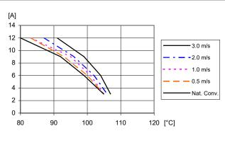
Available load current vs. ambient air temperature and airflow at Vo=5.0 V, VI = 12 V. See Thermal Consideration section.
