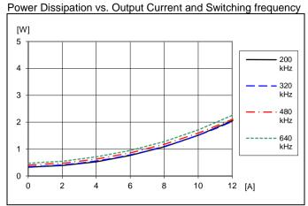
Dissipated power vs. load current and switching frequency at  $T_{P1} = +25^{\circ}C. V_1 = 12 V, V_{\Omega} = 3.3V, C_{\Omega} = 470 \mu F/10 m\Omega$ Default configuration except changed frequency
