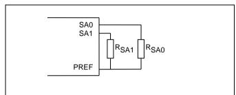
Schematic of connection of address resistor.
