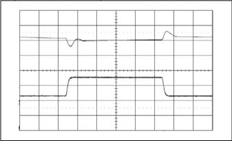
Output voltage response to load current stepchange (3-9-3 A) at:  $T_{P1} = +25^{\circ}C, V_1 = 12 V, V_0 = 3.3 V$ di/dt=2 A/µs, f\_sw=320 kHz, C\_0=470 µF/10 mΩ Default PID Control Loop and NLR
