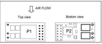
Temperature positions and air flow direction.
