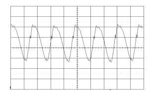
Output voltage ripple at: T<sub>P1</sub> = +25°C, Trace: output voltage (10 mV/div.).  $V_1 = 12 V, C_0 = 470 \mu F/10 m\Omega$ Time scale: (2 µs/div.) lo = 12 A
