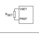
Using an external Pin-strap resistor,  $R_{SET}$ , the output voltage can be set in the range 0.6 V to 3.3 V at 28 different levels shown in the table below. The resistor should be applied between the VSET pin and the PREF pin.
