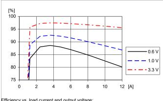
Efficiency vs. load current and output voltage: T<sub>P1</sub> = +25°C. V<sub>I</sub>=5 V, f<sub>sw</sub>=320 kHz, C<sub>0</sub>=470  $\mu$ F/10 mΩ.
