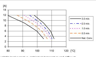
Available load current vs. ambient air temperature and airflow at  $V_0=5.0 \text{ V}$ ,  $V_1=12 \text{ V}$ . See Thermal Consideration section.
