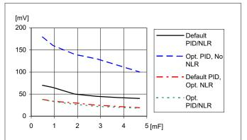
Load transient peak voltage deviation vs. external capacitance. Step-change (3-9-3 A). Parallel coupling of capacitors with 470  $\mu$ F/10 m $\Omega$ , T<sub>P1</sub> = +25°C. V<sub>I</sub>=12 V, V<sub>0</sub>=3.3 V, f<sub>sw</sub>=320 kHz, di/dt=2 A/µs
