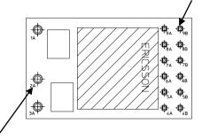
Pin 2A for measurement of minimum Pin (solder joint) temperature  $T_{\text{PIN}}$
