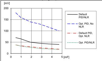
Load transient peak voltage deviation vs. decoupling capacitance. Step-change (3-9-3 A). Parallel coupling of capacitors with 470 μF/10 mΩ, T<sub>P1</sub> = +25°C. V<sub>1</sub>=12 V, V<sub>0</sub>=3.3 V, f<sub>sw</sub>=320 kHz, di/dt=2 A/µs
