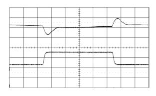
Output voltage response to load current step-change (3-9-3 A) at: +25°C, Vi = 12 V, Vo =3.3 V  $di/dt=2 A/us, f_{sw}=320 \text{ kHz}, C_0=470 \text{ }\mu\text{F}/10 \text{ }m\Omega$
