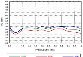
Input P0.1dB vs. Frequency at 5V over Temperature<sup>[1]</sup>
