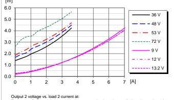
$T_{P1} = +25 \text{ °C}$ .  $I_{O1} = 0 \text{ A}$ ,  $V_1 = 53 \text{ V}$  when external voltage is supplied, no losses in main unit included for the curves when external voltage is supplied,
