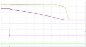
Yellow trace: DC/DC output voltage (5 V/div). Red trace: hold up voltage (20 V/div). Blue trace: input voltage (50 V/div). Green trace: Power Good (5 V/div). Time scale: (2 ms/div). Shutdown with default configuration for Power Good.
