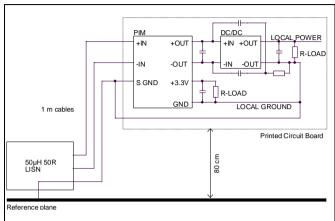
Conducted EMI Test set-up.
