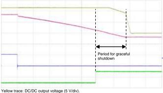
Yellow trace: DC/DC output voltage (5 V/div). Red trace: hold up voltage (20 V/div). Blue trace: input voltage (50 V/div). Green trace: Power Good (5 V/div). Time scale: (2 ms/div). Shutdown with Power Good in advance alert mode.
