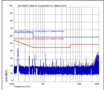
in combination with PKM 4613ANH  $V_l = 60 \text{ V}, \text{ C}_{01} = 330 \ \mu\text{F}$  electrolytic // 130  $\mu\text{F}$  ceramic,  $I_{01} \approx 10.5 \text{ A}$  $(I_{0\_DC/DC} = 50 \text{ A}), I_{02} = 3.6 \text{ A}$
