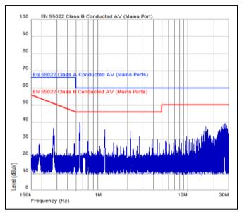
in combination with 2 x BMR 456 0004  $V_l = 48 \text{ V}, \text{ } C_{01} = 470 \text{ } \mu\text{F} \text{ electrolytic } // 30 \text{ } \mu\text{F} \text{ ceramic, } I_{01} \approx 17 \text{ A}$  $(I_{O_DC/DC} = 2 \times 32 \text{ A}), I_{O2} = 3.6 \text{ A}$
