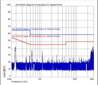
in combination with PKM 4817NH  $V_l = 53 V$ ,  $C_{01} = 330 \mu F$  electrolytic // 130  $\mu F$  ceramic,  $I_{01} \approx 17 A$  $(I_{0\_DCDC} \approx 75 A)$ ,  $I_{02} = 3.6 A$
