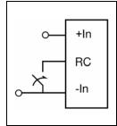
The product is fitted with a remote control function referenced to the primary negative input connection (-In). The RC function allows the product to be turned on/off by an external device like a semiconductor or mechanical switch. The RC pin has an internal pull up resistor to internal voltage reference 18V.
