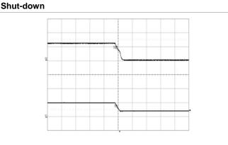
Shut-down enabled by disconnecting V<sub>1</sub> at:  $T_{P1} = +25^{\circ}C$ ,  $V_1 = 53 \text{ V}$ ,  $I_0 = 60 \text{ A resistive load}$ .
