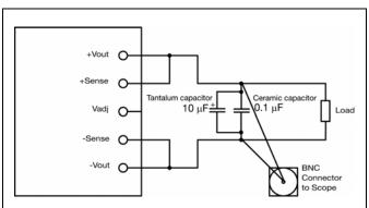
Output ripple and noise test setup
