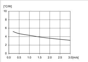
Thermal resistance vs. airspeed measured at the converter. Tested in wind tunnel with airflow and test conditions as per the Thermal consideration section.
