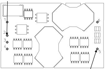
Pin 5 for measurement of minimum Pin (solder joint) temperature  $T_{PIN}$
