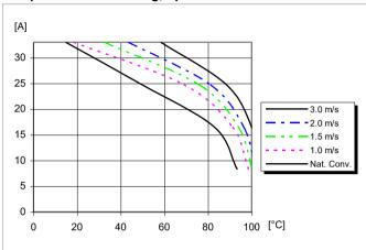
Available load current vs. ambient air temperature and airflow at V<sub>I</sub> = 53 V. See Thermal Consideration section.
