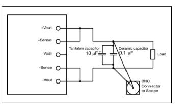
Output ripple and noise test setup
