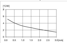
Thermal resistance vs. airspeed measured at the converter. Tested in wind tunnel with airflow and test conditions as per the Thermal consideration section. V<sub>I</sub> = 27 V.
