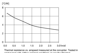
wind tunnel with airflow and test conditions as per the Thermal consideration section. V<sub>I</sub> = 27 V.
