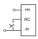
The products are fitted with a remote control function referenced to the primary negative input connection (-In), with negative and positive logic options available. The RC function allows the product to be turned on/off by an external device like a semiconductor or mechanical switch. The RC pin has an internal pull up resistor to +ln.
