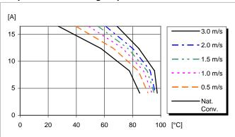
Available load current vs. ambient air temperature and airflow at  $V_{\rm I}$  = 27 V. See Thermal Consideration section.
