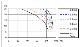
Available load current vs. ambient air temperature and airflow at  $V_1 = 27 \text{ V}$ . See Thermal Consideration section.
