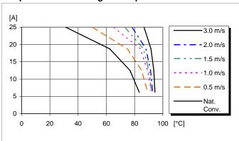
Available load current vs. ambient air temperature and airflow at  $V_1$  = 27 V. See Thermal Consideration section.
