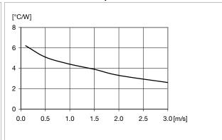
Thermal resistance vs. airspeed measured at the converter. Tested in wind tunnel with airflow and test conditions as per the Thermal consideration section.  $V_{\rm I}=27~\rm V.$
