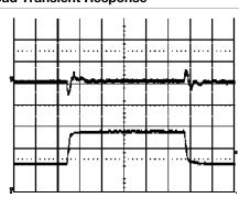
Output voltage response to load current step-change (30-60-30 A) at:  $T_{\rm ref}$  =+25°C,  $V_{\rm l}$  = 5.0 V.
