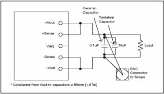
Output ripple and noise test setup
