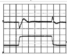
Output voltage response to load current stepchange (30-60-30 A) at: T<sub>ref</sub> =+25°C, V<sub>I</sub> = 5.0 V.
