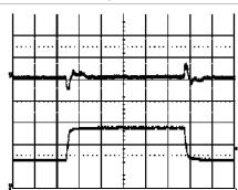
Output voltage response to load current step-change (30-60-30 A) at:  $T_{\rm ref}$  =+25°C,  $V_{\rm I}$  = 5.0 V.
