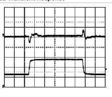
Output voltage response to load current stepchange (30-60-30 A) at:  $T_{ref}$  =+25°C,  $V_{l}$  = 5.0 V. Top trace: output voltage (100 mV/div.). Bottom trace: load current (20 A/div.). Time scale: 0.2 ms/div.
