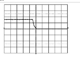
Shut-down enabled by disconnecting V<sub>i</sub> at:  $T_{ref} = +25^{\circ}\text{C}$ ,  $I_{O} = 60$  A resistive load,  $V_{I} = 5.0$  V.
