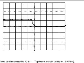
Shut-down enabled by disconnecting V, at:  $T_{\rm ref}=+25^{\circ}C,\,l_{O}=60$  A resistive load,  $V_{I}=5.0$  V.
