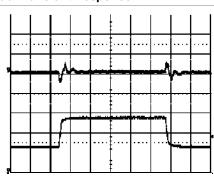
Output voltage response to load current step-change (30-60-30 A) at:  $T_{\rm ref}$  =+25°C, V<sub>I</sub> = 5.0 V.
