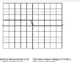
Shut-down enabled by disconnecting V, at:  $T_{ref}=+25^{\circ}C,\ l_{O}=60$  A resistive load,  $V_{i}=5.0$  V.
