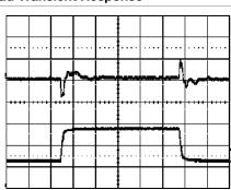
Output voltage response to load current stepchange (30-60-30 A) at: T<sub>ref</sub> =+25°C, V<sub>I</sub> = 3.3 V.
