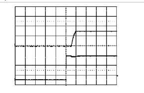
Start-up enabled by connecting V, at:  $T_{ref}$  = +25°C,  $I_{O}$  = 60 A resistive load,  $V_{I}$  = 5.0 V.
