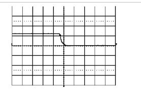
Shut-down enabled by disconnecting V  $_{\rm i}$  at:  $T_{\rm ref}=+25\,^{\circ}\text{C},\ I_{\rm O}=60$  A resistive load,  $V_{\rm I}=3.3$  V.
