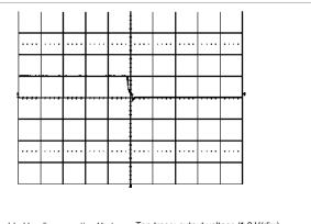
Shut-down enabled by disconnecting V  $_{\rm i}$  at:  $T_{\rm ref}=+25^{\circ}C,\ l_{O}=60$  A resistive load, V  $_{\rm i}=3.3$  V.
