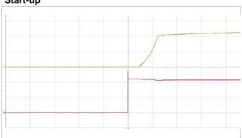
Start-up enabled by connecting  $V_{\text{I}}$  at:  $T_{P1}$  = +25 °C,  $V_{I}$  = 110 V,  $I_0 = 6.25$  A resistive load.
