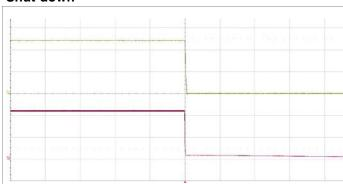
Shut-down enabled by disconnecting V<sub>I</sub> at:  $T_{P1} = +25 \, ^{\circ}\text{C}, \, V_{I} = 110 \, \text{V},$
