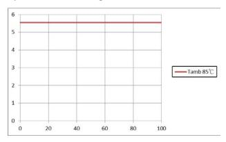
Available load current vs. cold wall temperature.  $V_{\text{I}}$  = 110 V. See Thermal Consideration section.
