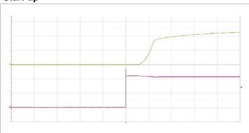
Start-up enabled by connecting  $V_{\text{I}}$  at: T<sub>P1</sub> = +25 °C, V<sub>I</sub> = 110 V,
