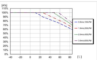
Available load current vs. ambient air temperature and airflow at  $V_1$  = 110 V with 0.79" heatsink. See Thermal Consideration section.
