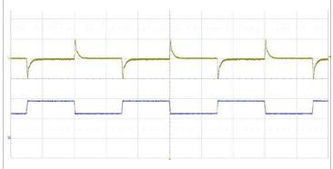
Output voltage response to load current step-change (6.25-9.375-6.35 A) at:  $T_{P1}$  = +25 °C,  $V_{I}$  = 110 V.
