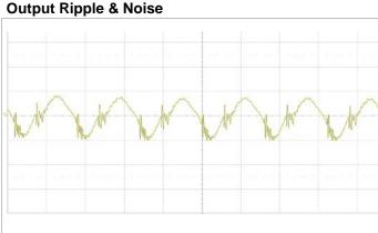
Output voltage ripple at: T<sub>P1</sub> = +25 °C, VI = 110 V,  $I_0 = 6.25$  A resistive load.
