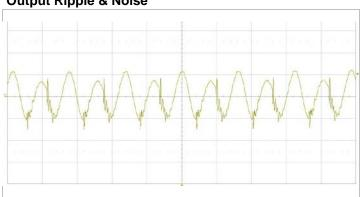
Output voltage ripple at: T<sub>P1</sub> = +25 °C, VI = 110 V,  $I_0$  = 12.5 A resistive load.
