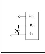
The products are fitted with a remote control function referenced to the primary negative input connection (-In), with negative and positive logic options available. The RC function allows the product to be turned on/off by an external device like a semiconductor or mechanical switch. The RC pin has an internal pull up resistor to +In.
