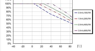
Available load current vs. ambient air temperature and airflow at  $V_1 = 110 \text{ V}$  with 0.5" heatsink. See Thermal Consideration section.
