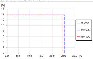
Output voltage vs. load current at  $I_0 > max I_0$  at +25 °C.
