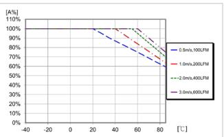
Available load current vs. ambient air temperature and airflow at  $V_1 = 110 \text{ V}$  with 0.79" heatsink. See Thermal Consideration section.
