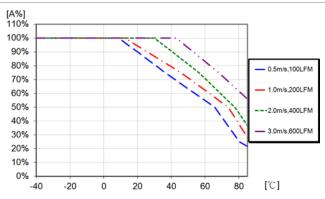
Available load current vs. ambient air temperature and airflow at  $V_{\rm l}$  = 110 V with 0.79" heatsink. See Thermal Consideration section.
