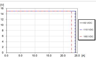
Output voltage vs. load current at  $I_0 > max I_0$  at +25 °C.
