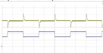
Output voltage response to load current step-change Top trace: output voltage (500 mV/div.). (3.125-4.6875-3.125 A) at:  $T_{P1} = +25 \, ^{\circ}\text{C}, \, V_{I} = 110 \, \text{V}.$
