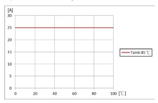
Available load current vs. cold wall temperature.  $V_{l}$  = 110 V. See Thermal Consideration section.
