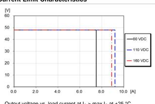
Output voltage vs. load current at  $I_0 > max I_0$  at +25 °C.
