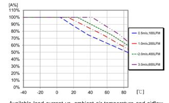
Available load current vs. ambient air temperature and airflow at  $V_1 = 110 \text{ V}$  with 0.5" heatsink. See Thermal Consideration section.
