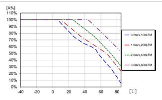
Available load current vs. ambient air temperature and airflow at  $V_{\rm l}=110~V$  with 0.5" heatsink. See Thermal Consideration section.
