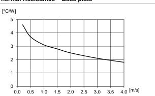
Thermal resistance vs. airspeed measured at the converter. Tested in wind tunnel with airflow and test conditions as per the Thermal consideration section.  $V_l = 53\ V.$
