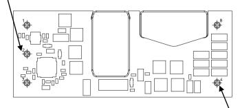
Pin 4 for measurement of minimum pin (solder joint) temperature, T<sub>PIN</sub>
