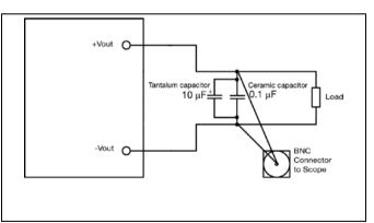
Output ripple and noise test setup
