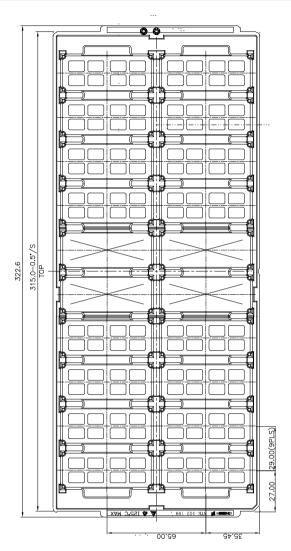
JEDEC standard tray for 2x10 = 20 products. All dimensions in mm [inch] Tolerances:  $X.x \pm 0.26$  [0.01],  $X.xx \pm 0.13$  [0.005] Note: pick up positions refer to center of pocket. See mechanical drawing for exact location on product.
