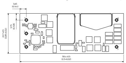
PIN SPECIFICATIONS Pin 1-4 & 8 Material: Copper alloy Plating: Min 0.1  $\mu m$  Au over 1-3  $\mu m$  Ni.
