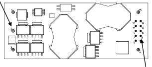
Pin 5 for measurement of minimum pin (solder joint) temperature,  $T_{PIN}$
