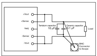
Output ripple and noise test setup
