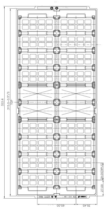
JEDEC standard tray for 2x5 = 10 products. All dimensions in mm [inch] Tolerances: X.x ±0.26 [0.01], X.xx ±0.13 [0.005] Note: pick up positions refer to center of pocket. See mechanical drawing for exact location on product.
