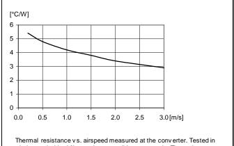
wind tunnel with airf low and test conditions as per the Thermal consideration section.  $V_{\rm I}$  = 53 V.
