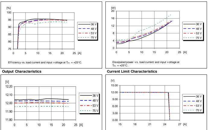
Output v oltage v s. load current at  $T_{P1}$  = +25°C.
