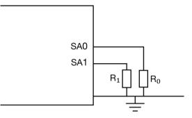
Schematic of connection of address resistors.
