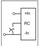
The device should be capable of sinking 0.7 mA. When the RC pin is left open, the voltage generated on the RC pin is max 6 V. The standard product is provided with "negative logic" remote control and will be off until the RC pin is connected to the -In. To turn on the product the voltage between RC pin and -In should be less than 1 V.
