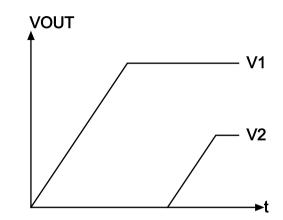
Illustration of Output Voltage Sequencing.
