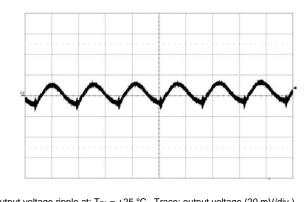
Output voltage ripple at: T<sub>P1</sub> = +25 °C, Trace: output voltage (20 mV/div.).  $V_1 = 12 V, C_0 = 470 \mu F/10 m\Omega$ Time scale: (2 µs/div.).  $I_{O} = 20 \text{ A}$
