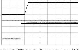
Start-up by enabling CTRL signal at:  $T_{P1} = +25 \text{ °C}, V_1 = 12 \text{ V}, V_0 = 1.0 \text{ V}$  $C_0 = 470 \ \mu\text{F}/10 \ \text{m}\Omega, \ I_0 = 25 \ \text{A}$
