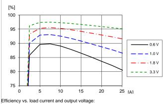
$T_{P1} = +25 \text{ °C}, V_1 = 5 \text{ V}, f_{sw} = 320 \text{ kHz}, C_0 = 470 \text{ }\mu\text{F}/10 \text{ m}\Omega.$
