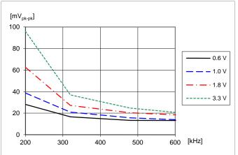
Output voltage ripple  $V_{pk\cdot pk}$  at:  $T_{P1}$  = +25 °C,  $V_{I}$  = 12 V,  $C_{O}$  = 470  $\mu F/10$  m $\Omega,$   $I_{O}$  = 25 A. Default configuration except changed frequency.
