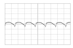
Output voltage ripple at: TP1 = +25 °C, Trace: output voltage (20 mV/div.).  $V_{I} = 12 V, C_{O} = 470 \ \mu\text{F}/10 \ \text{m}\Omega$  $I_{O} = 25 \text{ A}$ Time scale: (2 µs/div.).
