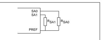
Schematic of connection of address resistor.
