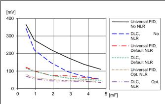
Load transient peak voltage deviation vs. decoupling capacitance. Step (6.25-18.75-6.25 A). Parallel coupling of capacitors with 470  $\mu F/10$  m\Omega, T<sub>P1</sub> = +25 °C. V<sub>1</sub> = 12 V, V<sub>0</sub> = 1.0 V, f<sub>sw</sub> = 320 kHz, di/dt = 2 A/µs
