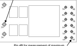
Pin 4B for measurement of maximum Product temperature T<sub>PRODUCT</sub>
