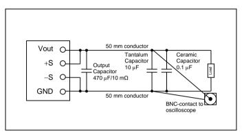
Output ripple and noise test set-up.
