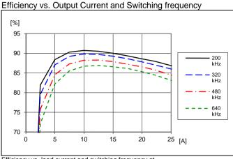
Efficiency vs. load current and switching frequency at  $T_{P1} = +25 \text{ °C}, V_1 = 12 \text{ V}, V_0 = 1.0 \text{ V}, C_0 = 470 \mu\text{F}/10 \text{ m}\Omega$ Default configuration except changed frequency
