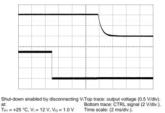
$T_{P1} = +25 \ ^{\circ}C, \ V_{I} = 12 \ V, \ V_{O} = 1.0 \ V \\ C_{O} = 470 \ \mu F/10 \ m\Omega, \ I_{O} = 25 \ A$ Time scale: (2 ms/div.).
