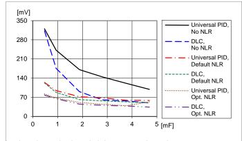
Load transient peak voltage deviation vs. external capacitance. Step (6.25-18.75-6.25 A). Parallel coupling of capacitors with 470  $\mu$ F/10 m $\Omega$ , T<sub>P1</sub> = +25 °C. V<sub>1</sub> = 12 V, V<sub>0</sub> = 1.0 V, f<sub>sw</sub> = 320 kHz, di/dt = 2 A/ $\mu$ s
