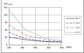
Output voltage ripple V<sub>pk-pk</sub> at:  $T_{P1}$  = +25 °C, V<sub>1</sub> = 12 V, C<sub>0</sub> = 470 µF/10 mΩ, Io = 25 A resistive load. Default configuration except changed frequency.
