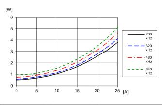
Dissipated power vs. load current and switching frequency at  $T_{P1} = +25 \text{ °C}, V_1 = 12 \text{ V}, V_0 = 1.0 \text{ V}, C_0 = 470 \text{ }\mu\text{F}/10 \text{ m}\Omega$ Default configuration except changed frequency
