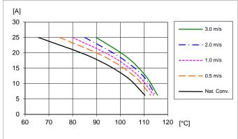
Available load current vs. ambient air temperature and airflow at  $V_0 = 1.0 V$ ,  $V_1 = 12 V$ . See Thermal Consideration section
