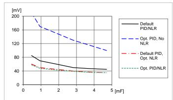
Load transient peak voltage deviation vs. external capacitance. Step-change (5-15-5 A). Parallel coupling of capacitors with 470  $\mu$ F/10 m $\Omega$ , T<sub>P1</sub> = +25 °C, V<sub>1</sub>= 12 V, V<sub>0</sub> = 1.0 V, f<sub>sw</sub> = 320 kHz, di/dt = 2 A/ $\mu$ s
