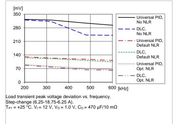
Note 1: For Universal PID, see section Dynamic Loop Compensation (DLC).
