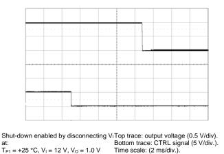
at:  $T_{P1} = +25 \text{ °C}, V_1 = 12 \text{ V}, V_0 = 1.0 \text{ V}$   $C_0 = 470 \text{ }\mu\text{F}/10 \text{ }m\Omega, I_0 = 20 \text{ A}$ Time scale: (2 ms/div.).
