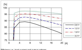
Efficiency vs. load current and output voltage:  $T_{P1} = +25 \text{ }^{\circ}\text{C}, V_1 = 5 \text{ } V, f_{sw} = 320 \text{ } \text{kHz}, C_0 = 470 \text{ } \mu\text{F}/10 \text{ } \text{m}\Omega.$
