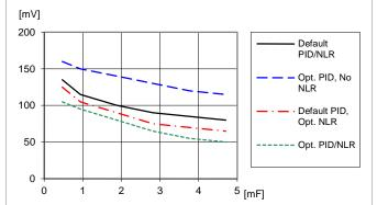
Load transient peak voltage deviation vs. external capacitance. Step-change (5-15-5 A). Parallel coupling of capacitors with 470  $\mu$ F/10 m $\Omega$ , T<sub>P1</sub> = +25 °C, V<sub>1</sub>= 12 V, V<sub>0</sub> = 3.3 V, f<sub>sw</sub> = 320 kHz, di/dt = 2 A/ $\mu$ s
