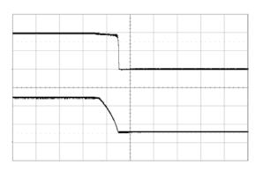
Shut-down enabled by disconnecting V<sub>I</sub> at: T<sub>P1</sub> = +25 °C, V<sub>I</sub> = 12 V, V<sub>O</sub> = 1.0 V  $C_0 = 470 \ \mu F / 10 \ m \Omega$ ,  $I_0 = 20 \ A$
