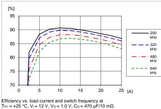
TP1 = +25 °C, V1 = 12 V, V0 = 1.0 V, C0 = 470  $\mu$ F/10 m $\Omega$ Default configuration except changed frequency
