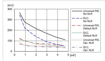
Load transient peak voltage deviation vs. external capacitance. Step (6.25-18.75-6.25 A). Parallel coupling of capacitors with 470  $\mu$ F/10 mΩ, T<sub>P1</sub> = +25 °C, V<sub>1</sub>= 12 V, V<sub>0</sub> = 1.0 V, f<sub>sw</sub> = 320 kHz, di/dt = 2 A/ $\mu$ s
