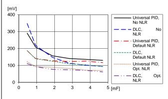
Load transient peak voltage deviation vs. decoupling capacitance. Step (6.25-18.75-6.25 A). Parallel coupling of capacitors with 470  $\mu F/10$  m\Omega,  $T_{P1} = +25 \text{ °C. } V_1 = 12 \text{ V}, V_0 = 3.3 \text{ V}, f_{sw} = 320 \text{ kHz}, di/dt = 2 \text{ A}/\mu\text{s}$
