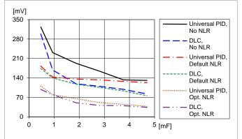
Load transient peak voltage deviation vs. external capacitance. Step (6.25-18.75-6.25 A). Parallel coupling of capacitors with 470  $\mu$ F/10 m $\Omega$ , T<sub>P1</sub> = +25 °C. V<sub>1</sub> = 12 V, V<sub>0</sub> = 3.3 V, f<sub>sw</sub> = 320 kHz, di/dt = 2 A/ $\mu$ s
