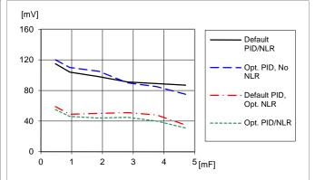
Load transient peak voltage deviation vs. external capacitance. Step-change (5-15-5 A). Parallel coupling of capacitors with 470  $\mu$ F/10 m $\Omega$ , T<sub>P1</sub> = +25 °C, V<sub>1</sub>= 12 V, V<sub>0</sub>= 3.3 V, f<sub>sw</sub> = 320 kHz, di/dt = 2 A/ $\mu$ s
