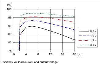
T<sub>P1</sub> = +25 °C, V<sub>I</sub> = 5 V, f<sub>sw</sub> = 320 kHz, C<sub>0</sub> = 470  $\mu$ F/10 mΩ.
