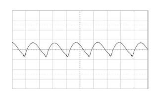
Output voltage ripple at: TP1 = +25 °C, Trace: output voltage (10 mV/div.).  $V_1 = 12 V, C_0 = 470 \mu F/10 m\Omega$ Time scale: (2 µs/div.).  $I_{O} = 20 \text{ A}$
