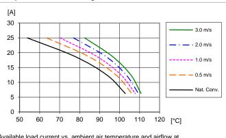
Available load current vs. ambient air temperature and airflow at  $V_0 = 3.3 V$ ,  $V_1 = 12 V$ . See Thermal Consideration section.
