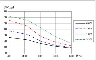
Output voltage ripple  $V_{pk\cdot pk}$  at:  $T_{P1}$  = +25 °C,  $V_I$  = 12 V,  $C_O$  = 470  $\mu F/10$  m $\Omega,$   $I_O$  = 20 A. Default configuration except changed frequency.
