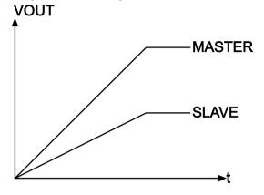
Illustration of Ratiometric Voltage Tracking
