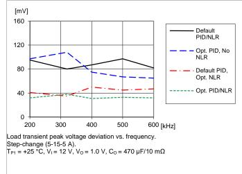
Note: In the load transient graphs, the worst-case scenario (load step 15-5 A) has been considered.
