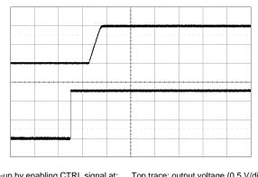
Start-up by enabling CTRL signal at: T\_{P1} = +25 ~^{\circ}C, V\_{I} = 12 ~V, V\_{O} = 1.0 ~V C\_{O} = 470  $\mu F/10~m\Omega,~I_{O} = 25~A$
