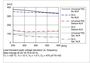
Note 1: For Universal PID, see section Dynamic Loop Compensation (DLC). Note 2: In the load transient graphs, the worst-case scenario (load step 18.75-6.25 A) has been considered.
