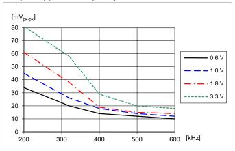
Output voltage ripple V<sub>pk·pk</sub> at: T<sub>P1</sub> = +25 °C, V<sub>I</sub> = 12 V, C<sub>O</sub> = 470  $\mu$ F/10 m $\Omega$ ,  $I_0$  = 20 A. Default configuration except changed frequency.
