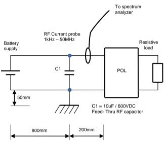
Conducted EMI test set-up
