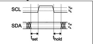
Setup and hold times timing diagram
