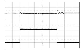
Output voltage response to load current step-change (6.25-18.75-6.25 A) at: T<sub>P1</sub> = +25 °C, V<sub>1</sub> = 12 V, V<sub>0</sub> = 1.0 V di/dt=2 A/µs, f<sub>sw</sub> = 320 kHz, C<sub>0</sub> = 470 µF/10
