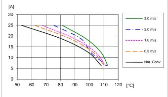
Available load current vs. ambient air temperature and airflow at Vo = 1.0 V, VI = 12 V. See Thermal Consideration section.
