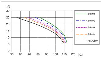
Available load current vs. ambient air temperature and airflow at Vo = 0.6 V, VI = 12 V. See Thermal Consideration section.
