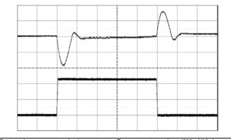
Output voltage response to load current stepchange (6.25-18.75-6.25 A) at: T<sub>P1</sub> = +25 °C, V<sub>I</sub> = 12 V, V<sub>O</sub> = 1.0 V di/dt=2 A/µs, f<sub>sw</sub> = 320 kHz, C<sub>0</sub> = 470 µF/10 mΟ DLC and no NLR
