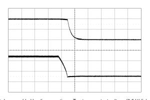
Shut-down enabled by disconnecting Vi at:  $T_{P1} = +25 \text{ °C}, V_I = 12 \text{ V}, V_O = 1.0 \text{ V}$  $C_0 = 470 \ \mu F/10 \ m\Omega$ ,  $I_0 = 25 \ A$
