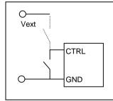
The product is equipped with a remote control function, i.e., the CTRL pin. The remote control can be connected to either the primary negative input connection (GND) or an external voltage (Vext), which is a 3 - 5 V positive supply voltage in accordance to the SMBus Specification version 2.0.
