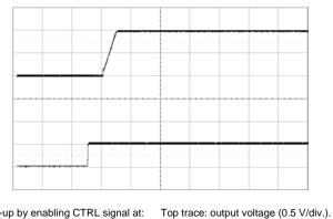
Start-up by enabling CTRL signal at: T\_P1 = +25 °C, V\_I = 12 V, V\_0 = 1.0 V C\_0 = 470 \ \mu\text{F}/10 \ \text{m}\Omega, \ I\_0 = 20 \ \text{A}
