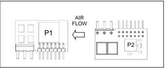
Temperature positions and air flow direction.
