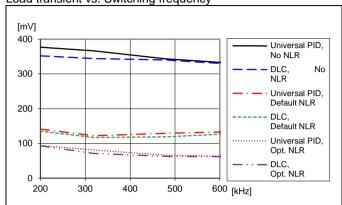
Load transient peak voltage deviation vs. frequency. Step-change (6.25-18.75-6.25 A). TP1 = +25 °C, V<sub>1</sub> = 12 V, V<sub>0</sub> =1.0 V, C<sub>0</sub> = 470 μF/10 mΩ
