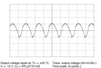
$V_1 = 12 V, C_0 = 470 \mu F/10 m\Omega$  $I_{0} = 25 \text{ A}$
