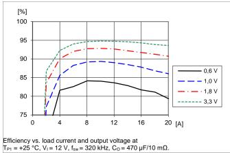
Efficiency vs. Output Current and
