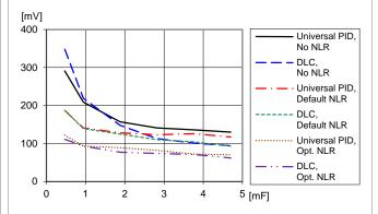
Load transient peak voltage deviation vs. external capacitance. Step (6.25-18.75-6.25 A). Parallel coupling of capacitors with 470  $\mu$ F/10 mΩ, T<sub>P1</sub> = +25 °C, V<sub>1</sub> = 12 V, V<sub>0</sub> = 3.3 V, f<sub>sw</sub> = 320 kHz, di/dt = 2 A/µs
